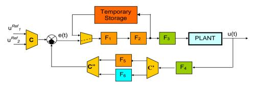
Fig. 3. Control system pipeline
