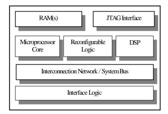
Fig. 1. Possible structure of a future Field Configurable System on a Chip
