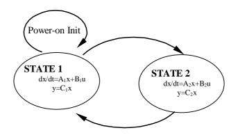
Fig. 3. The state transition graph of the re-configurable controller
