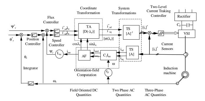
Fig. 4. State 1: Vector control system for voltage-source inverter-fed induction machine
