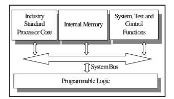
Fig. 2. Structure of the Triscend CSoC
