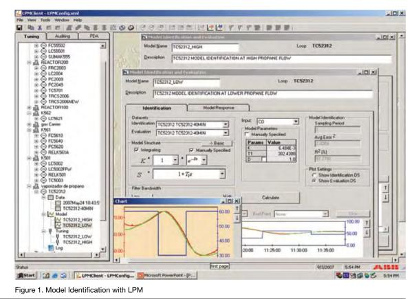
Figures 1 and 2 show different steps of the tuning process using LPM. Control engineers appreciated the full functionality of the ABB loop tuning software, especially the ability to create process models. The control engineers found LPM very useful. Consider the LPM application on a distillation column and heat exchanger. Single loops were tuned primarily with the Lambda method for simple loops, and Dominant Pole Placement for complex ones.
