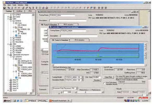
Figure 2. Loop Tuning and Evaluation with LPM
