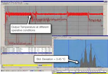
Figures 3 and 4 show different trends and standard deviations of the output temperature of a heat exchanger before and after the PID controllers were tuned with the ABB LPM.
