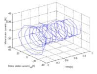
Fig. 10. Motor current stator space phasor
