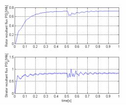
Fig. 6. Rotor and stator resultant flux.
