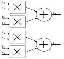
Fig. 7. Universal computation module of vector control systems
