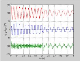
Fig. 4. Current waveforms before and after reconfiguration. It can be observed that the reconfiguration introduces perturbations in every observed parameter of the drive (Fig. 5 and Fig. 6).
