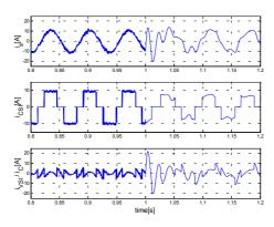
Fig. 9. Simulated current waveforms before and after reconfiguration.
